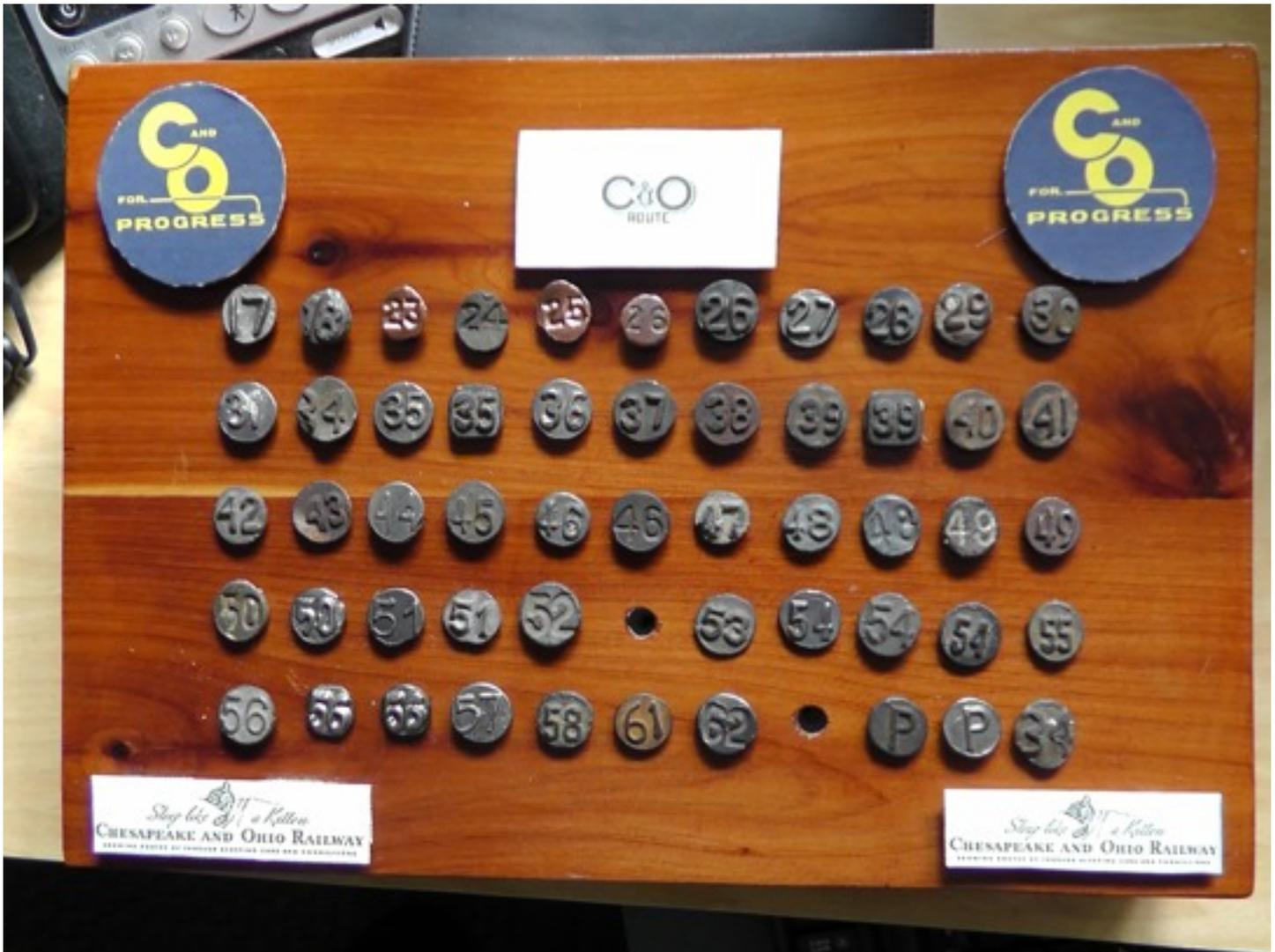
Railroads in the U.S. no longer use date nails. With the advent of the computer it is easier to keep records that way. Also, the treatments are pretty much fine tuned and standardized at this point. It must also be noted that several railroads have replaced wooden ties with composite or concrete ones. It is hard to drive a date nail into a concrete tie! 1969 was the last hurrah for date nails used by major railroads in the U.S.
