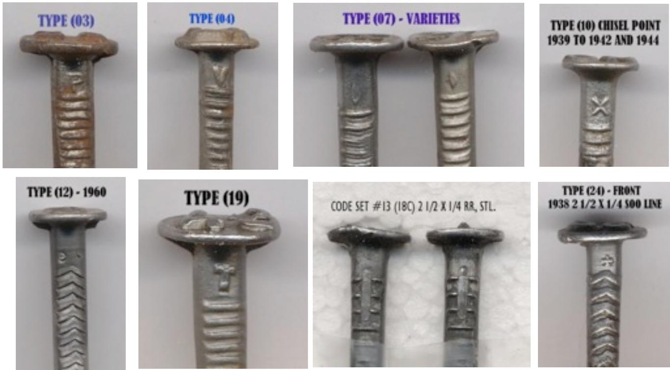
In other words, all the nails with the “P” under the head came from one manufacturer, in this case the Pittsburgh Steel Company. The ones with the “V” on the shank under the head were manufactured by the Republic Steel Corp.
