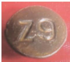
Along with the date nails there were special treatment nails made that showed the type of treatment - such as the Milwaukee Road Z 9 - which indicated a zinc tie treated in 1909 or the Great Northern F 4 which indicated it was a Fir tie that was treated in 1904.
